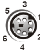
Figure B-4. Pin Numbers for the Keyboard Connector
